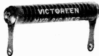
Victoreen 210 M\Omega resistor from the HV series.
